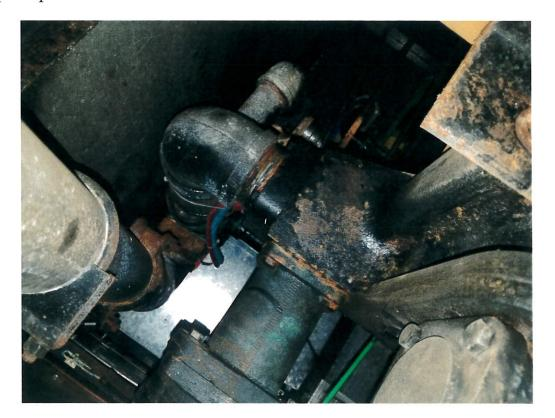
Frame- This is an area of serious concern, this truck has seen duty for 25 winters in New Hampshire and been exposed to road treatment chemicals. The frame shows signs of rust and based on my experience if left unrepaired the frame will be damaged beyond repair in just a few more years. The white powder on the frame in these photos is road treatment that has worked it's way between the truck frame and body frame, both of which are untreated metal.
