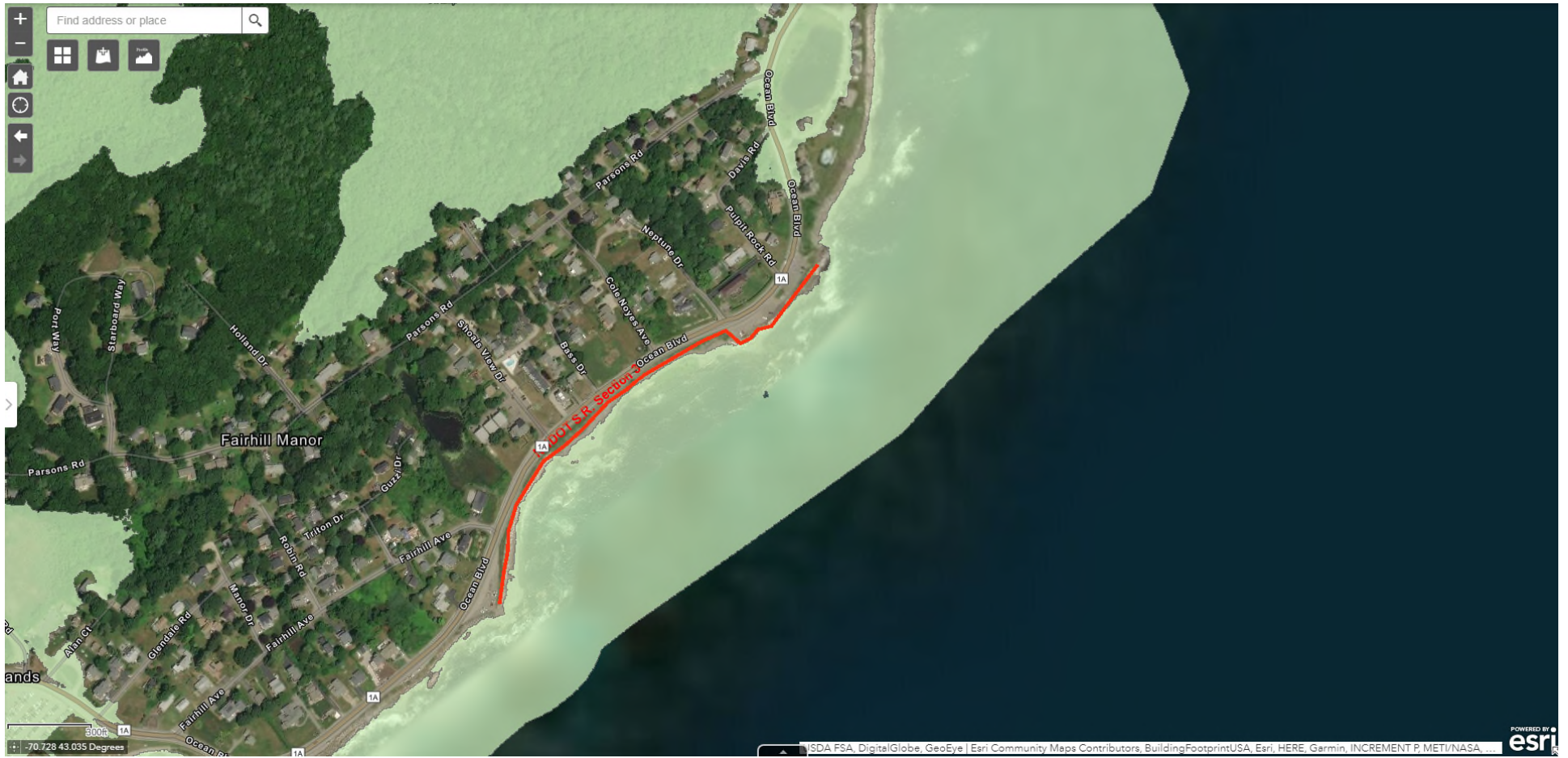
Figure 22. Flood inundation at Stillwater Elevation 8.5 feet NAVD88 – Vicinity of Section 3.
