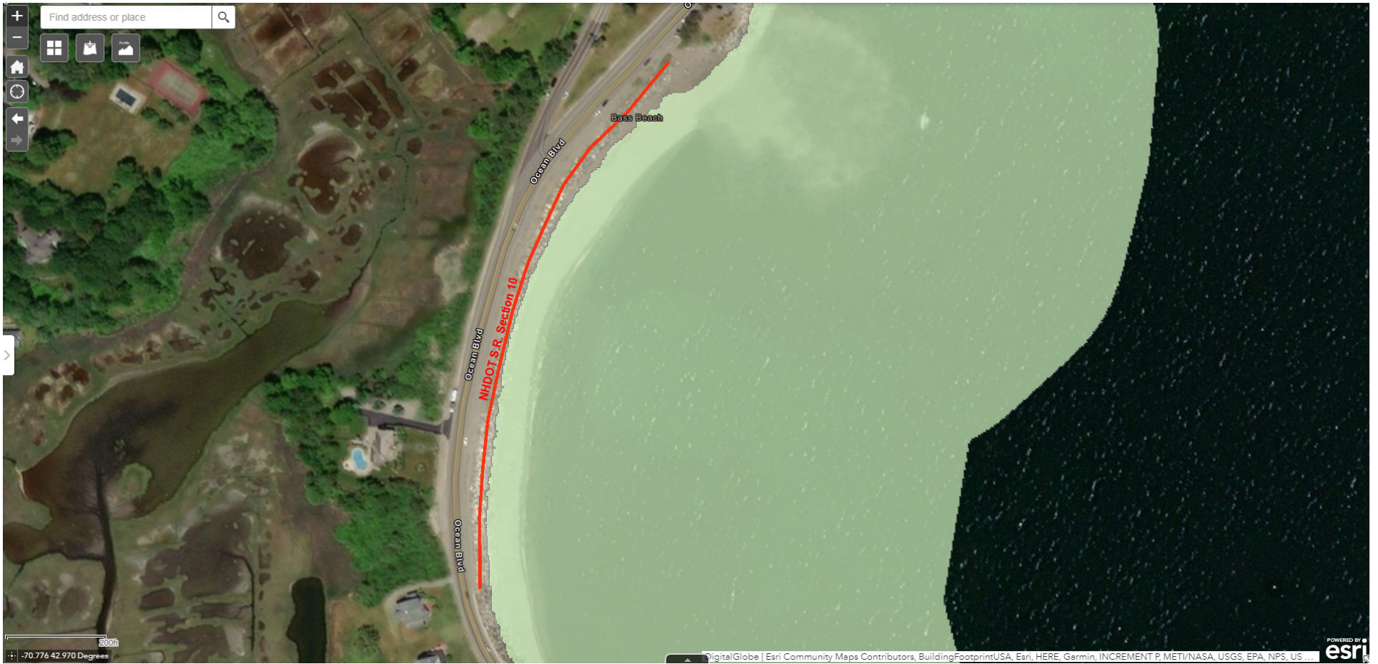
Figure 52. Flood inundation at Stillwater Elevation 8.5 feet NAVD88 – Vicinity of Section 10.
