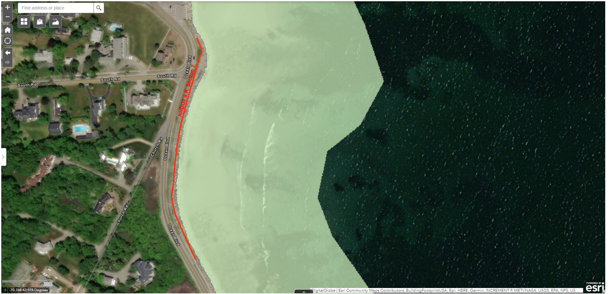
Figure 46. Flood inundation at Stillwater Elevation 8.5 feet NAVD88 – Vicinity of Section 7.
