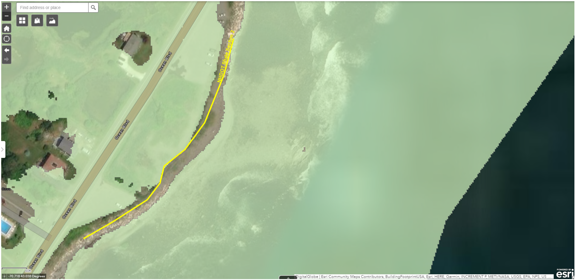
Figure 16. Flood inundation at Stillwater Elevation 8.5 feet NAVD88 – Vicinity of Section 2.
