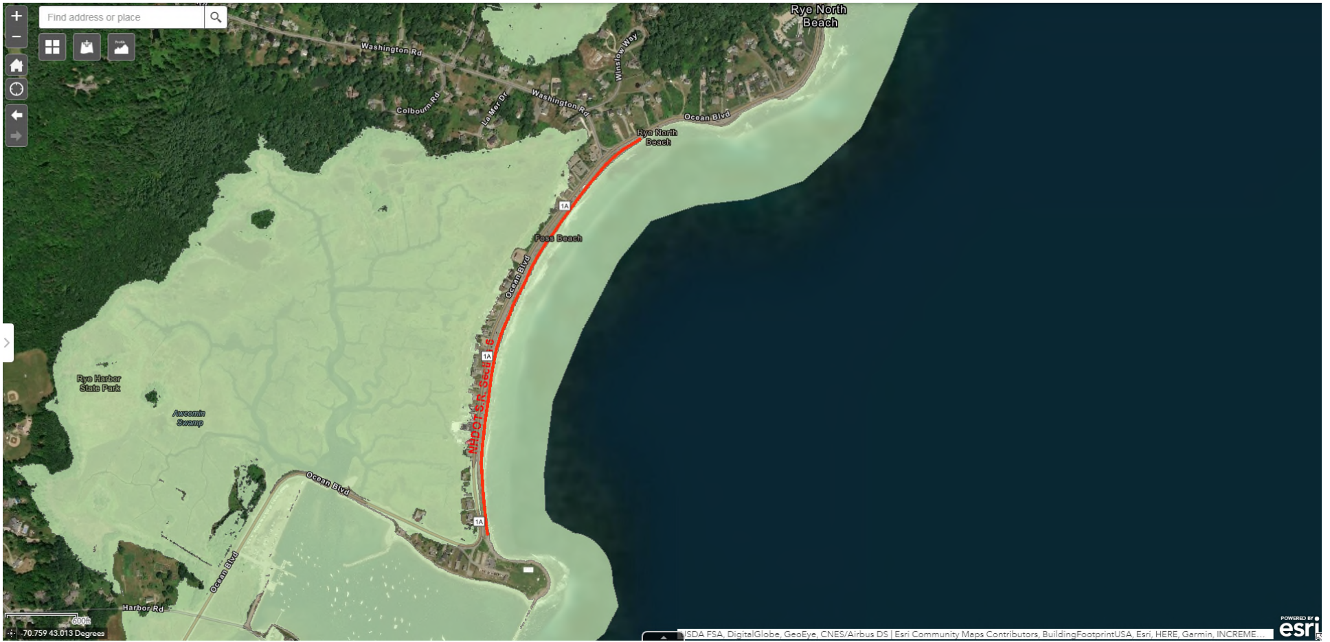
Figure 40. Flood inundation at Stillwater Elevation 8.5 feet NAVD88 – Vicinity of Section 6.
