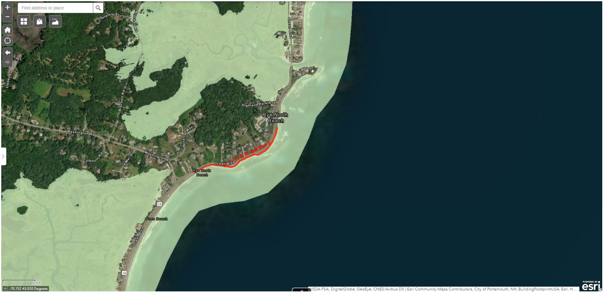
Figure 34. Flood inundation at Stillwater Elevation 8.5 feet NAVD88 – Vicinity of Section 5.
