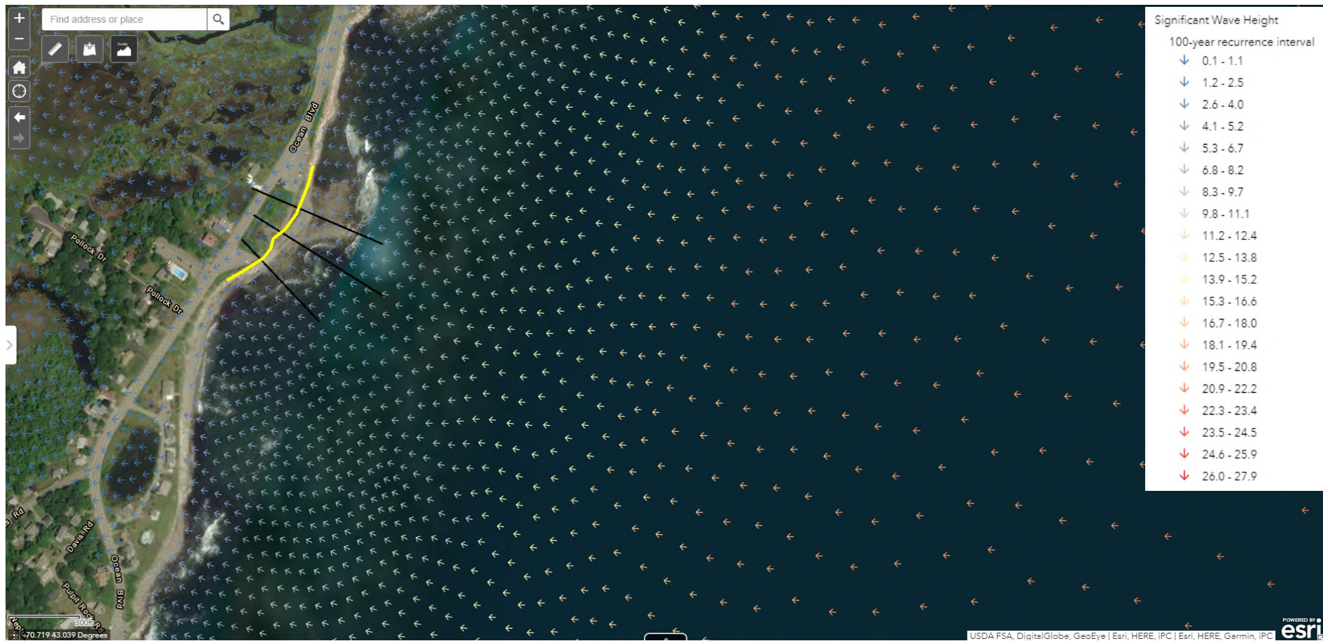
Figure 18. 100-year Recurrence Interval Wave Height (feet) for Transect 1, 2, 3 at NHDOT S.R. Section 2.
